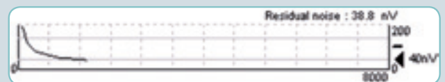
Rather than testing for a certain number of sweeps, the residual noise should be used as a stop criteria.
